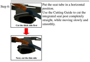
**A** CAUTION: To avoid fraying the composite fibers. Using a fine tooth (32 teeth) saw blade is recommended.
